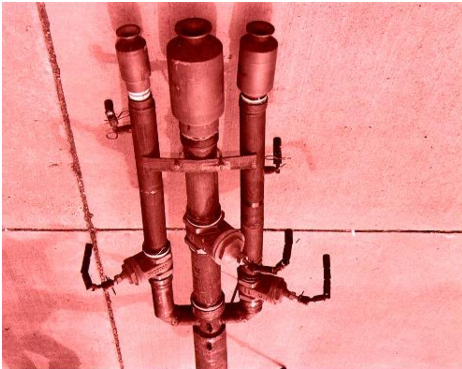
Figure 2. Three Nozzles and Movable Header Manifold Used in Tests
