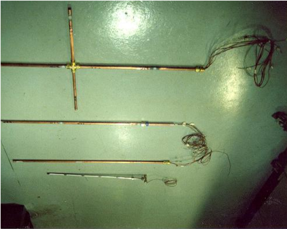
Figure 5. Temperature Measurement Devices (Bottom Side View)
