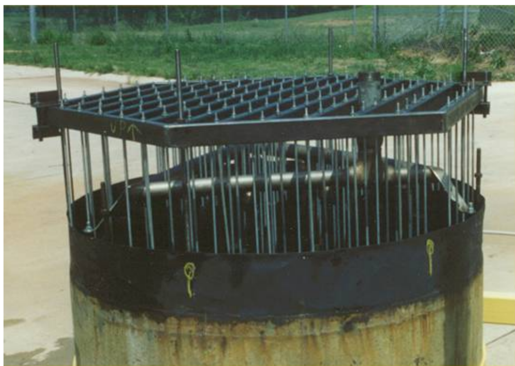
Figure 2. F.R.I. Adjustable Liquid Distributor
